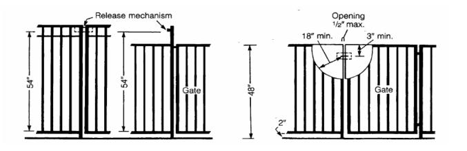
The release mechanism shall be located at 54" or higher from the bottom of the gate.
