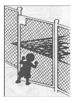
These are the gates people must walk through. Swimming pool barriers should be equipped with a gate or gates which restrict access to the pool. A locking device must be included in the gate design. Pedestrian gates must open outward and away from the pool and shall be self-closing and self-latching.
