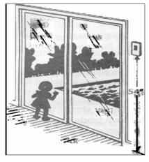
1) All doors which give direct access to a swimming pool must be equipped with an audible alarm which sounds when the door and/or screen are opened. The alarm must sound for 30 seconds or more immediately after the door is opened. The alarm must be capable of being heard throughout the house during normal household activity. (The alarm sound should be distinct from other sounds in the house, such as the telephone, doorbell and smoke alarm.) The alarm must have an automatic reset feature.
