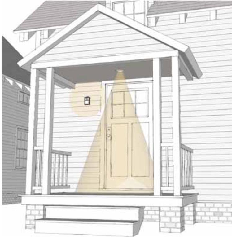
Small surface mounted or ceiling mounted exterior lights located within the porch area are the most appropriate fixtures for Truxtun.
